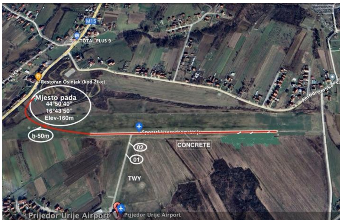
Picture 1.1: The aircraft's path, accident's site and locations of eyewitnesses
