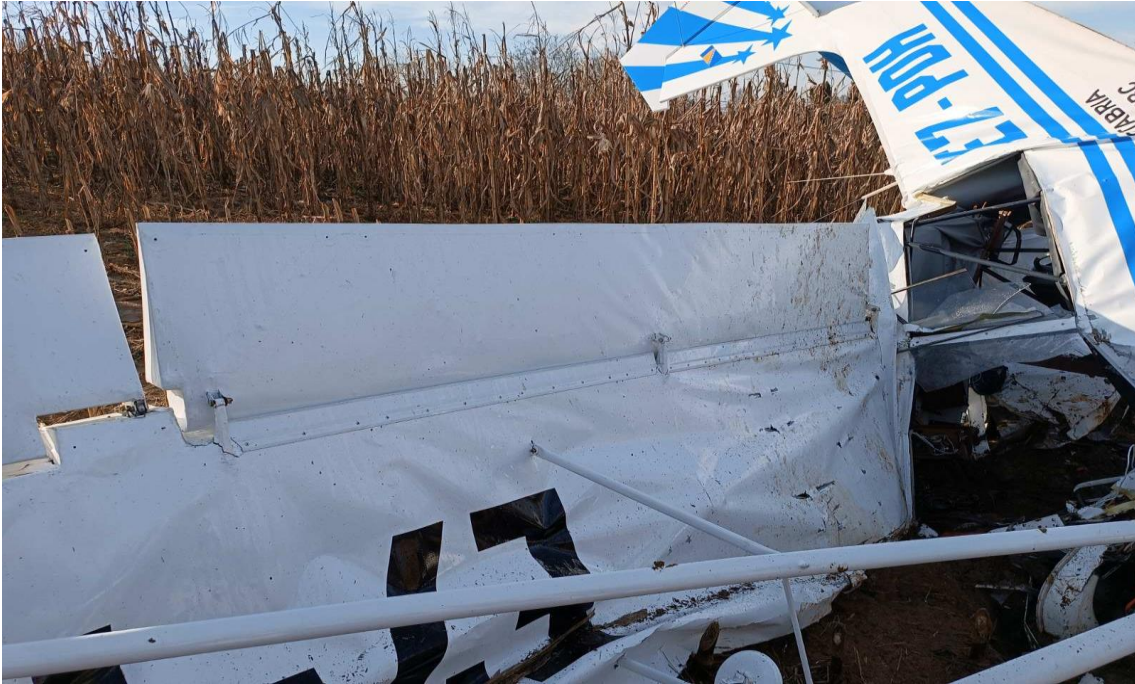
Picture number 1.7: Left wing and flap in retracted position
