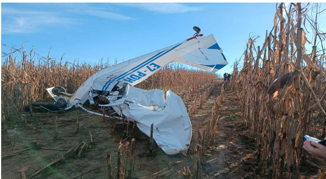
Picture no. 1.5: Position of aircraft after hitting the ground (the right side)
