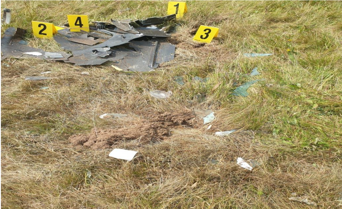
Figure 1.10: First impact into the ground, engine case debris, a propeller blade and parts of plexiglass
