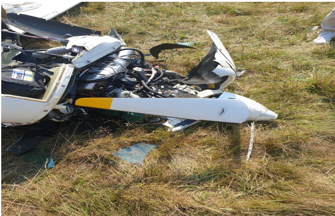
Figure 1.11 Plane's nose, engine, proppeler hub and proppeler blade after the accident
